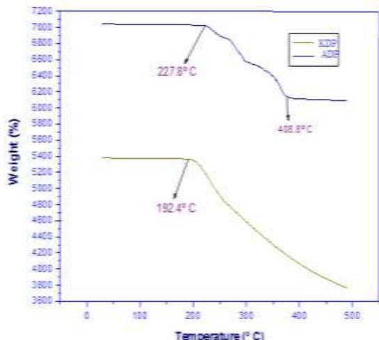
Fig. 6a TGA thermogram of KDP and ADP crystals
