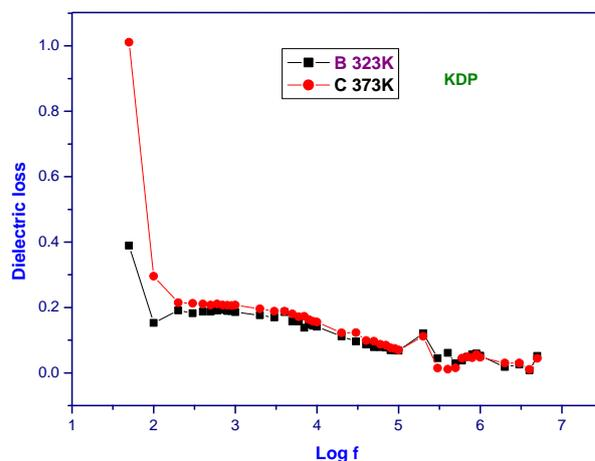
Fig. 5c Log f vs Dielectric loss of KDP crystals
