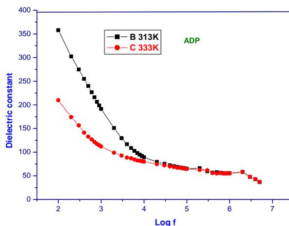
Fig. 5b Log f vs Dielectric constant of ADP crystals
