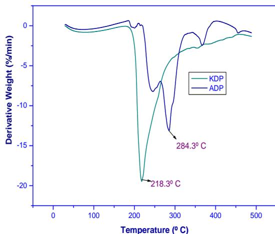
Fig. 6b DTA thermogram of KDP and ADP crystals
