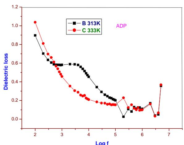
Fig. 5d Log f vs Dielectric loss of ADP crystals
