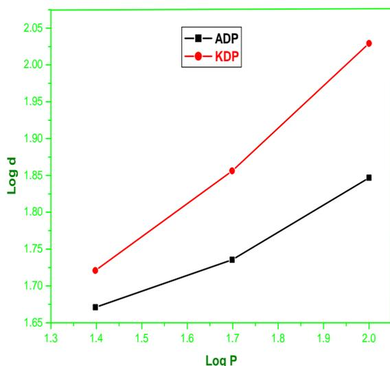
Fig. 4 b. Log P Vs Log d for KDP and ADP single crystal
