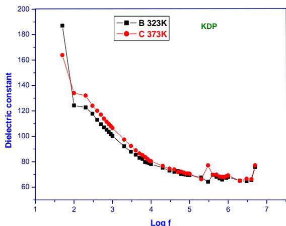
Fig. 5a Log f vs Dielectric constant of KDP crystals
