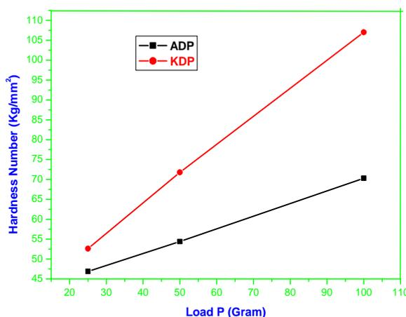
**Fig. 4 a. Load P Vs Hardness Number for KDP and ADP single crystal**
